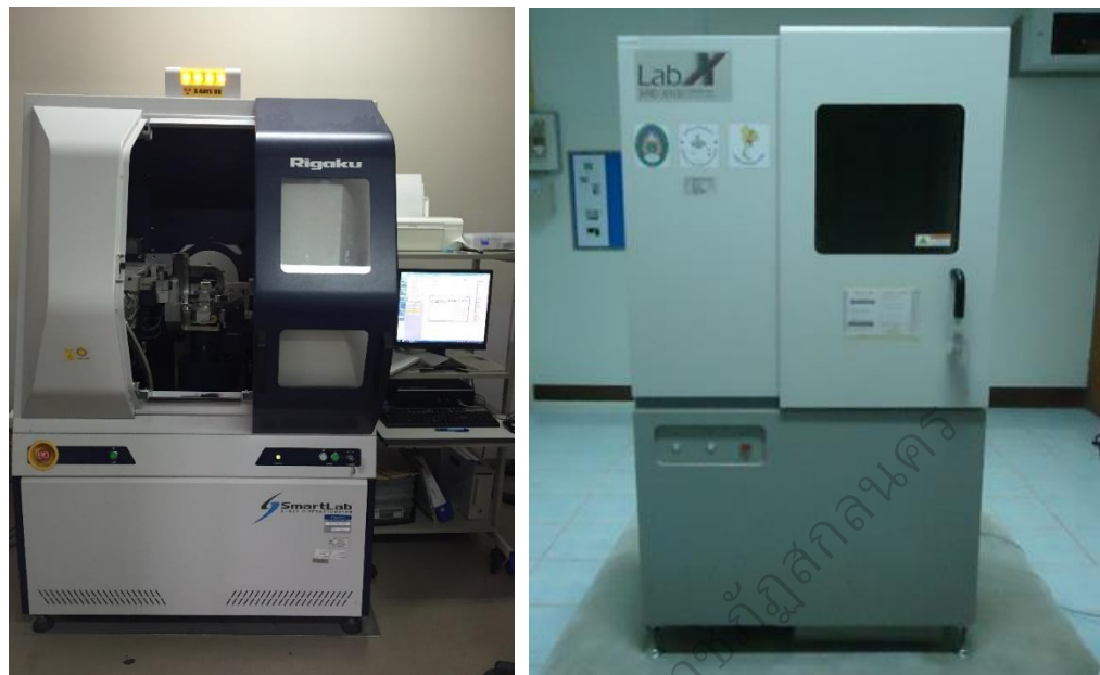
Figure 12 the X-ray diffraction (XRD) measurements was performed on (left) Rigaku Smart Lab at Osaka Prefecture University and (right) Center of Excellence on Alternative Energy at Sakon Nakhon Rajabhat University
