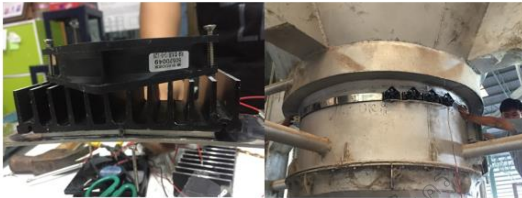
Figure 48 Show thermogenerator machine for install on stove fuel of rice dryer Machine
