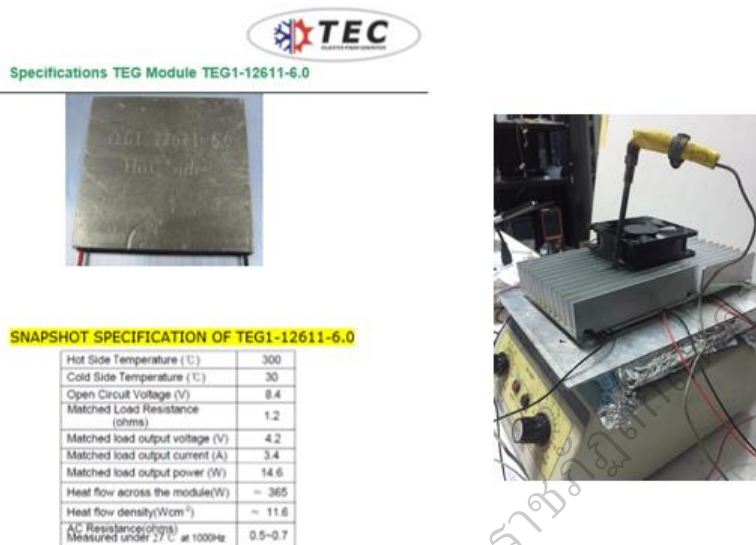
Figure 46 Show thermoelectric module from TEC Thermoelectric gencell technology and process of analyzed performance of 6–8 module by setting system on laboratory
