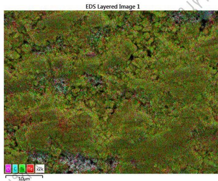
Figure 46 Mapping of \text{Bi}_2\text{Te}_3 bulk
