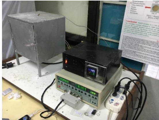
Figure 25 the measurement was carried out by Chen Hwa 1061 LCR-Meter.
