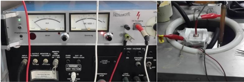
Figure 26 A polling quantity of 6 kV per 1 mm thickness of PVDF, which must be polled at least 0.12 kV potential difference. In the experiment, the polls at 1.5 kV with PVDF-CNT poles ranged from 0% to 5%.
