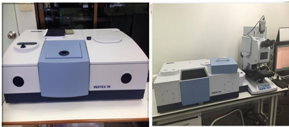
Figure 24 Fourier Transform InfraRed Spectrometer(FT-IR) is an instrument used for the analysis of the functional group of organic compounds. Based on the principle of absorption of the middle infrared region, about 400\text{-}4000\text{ cm}^{-1} .
