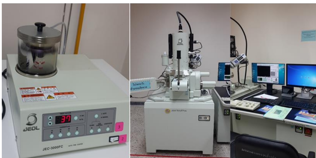
Figure 23 Scanning Electron Microscope (SEM) is an electron microscope. Imaging is performed by measuring the electrons reflected from the surface of the surveyed samples.
