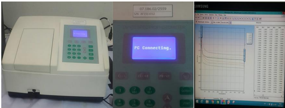
Figure 25 UV-VIS Spectrophotometer It is an instrument used in the analysis of substances based on the radiation absorption principle of substances in the range of Ultra violet (UV) and Visible (VIS) wavelength about 190-1000 nm.
