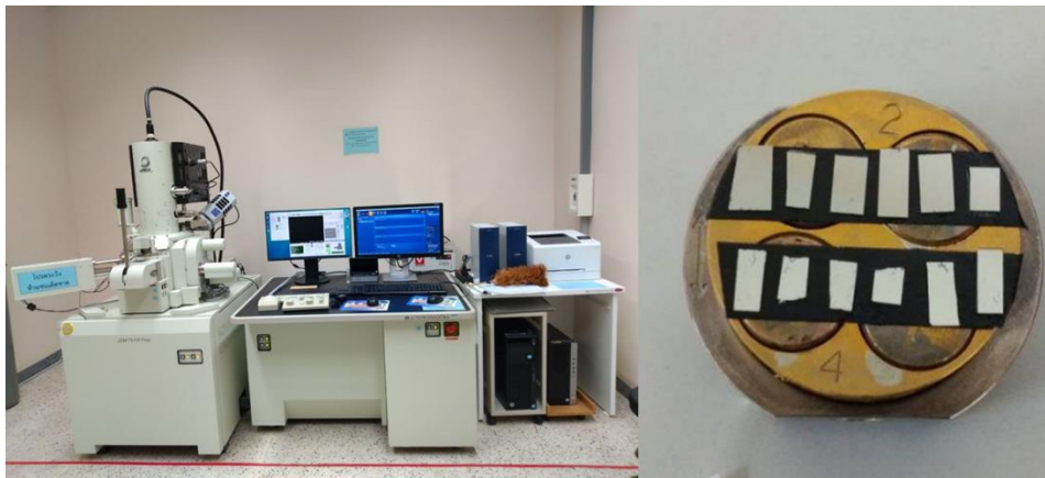
Figure 26 Field emission scanning electron microscopy JSM-7610FPlus, JEOL (FE-SEM) of Ubon ratchathani university and preparation of Ag-Doped \text{Sb}_2\text{Te}_3 thin films.
