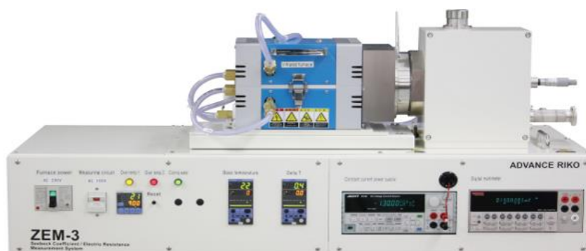
Figure 27 Seebeck Coefficient/Electric Resistance Measurement System ZEM-3 series at center of excellence on alternative energy sakon nakhon rajabhat university.
